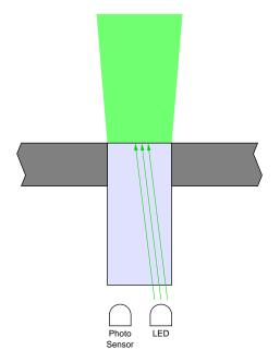
Fig. 8: Light Cone of a standard Light Guide Setup
