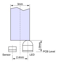
Fig. 5: Mechanical Dimensions of the Setup
