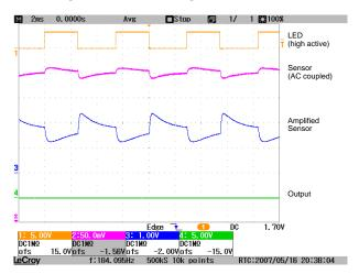
Fig. 11: Waveforms of a non-activated Button
