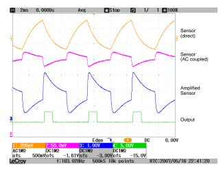
Fig. 12: Waveforms of an activated Button
