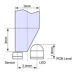
Fig. 10: Mechanical Dimensions of the beveled Setup
